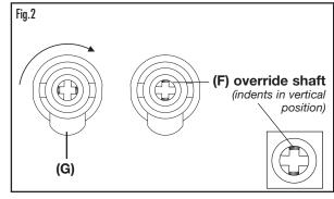
3. Push the lever catch (G) in to be flush with drive tube (E) diameter. Now the lock is ready to receive outside lever assembled with cylinder(B) (see fig. 3)
