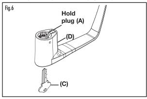
7. The key (C) must be in the horizontal position as shown below
